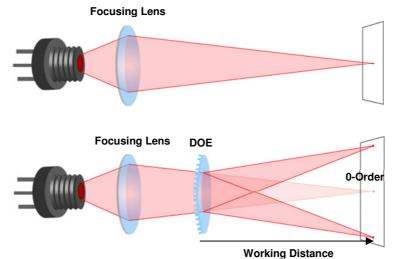
Laser diodes are the most common light source to be used with diffractive optical elements, but other laser light sources may also be used.
